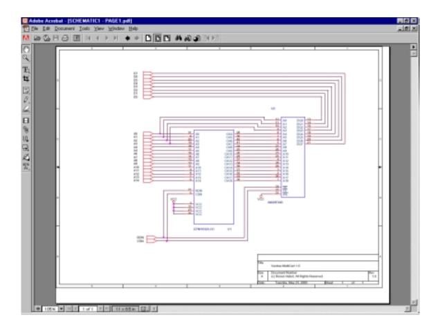
The following schematic represents the content of the EPLD device.
