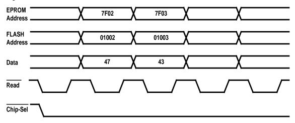
In this case, the address is correct, but, the data read from the Flash is part of the Vectrex header that must be present at the beginning of each game (in this case the letters GC that are part of the "© GCE
