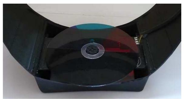
**Fig. 3** View inside the 3d Imager, showing the colour wheel and placement of so called "calibration" wheel/ring.
